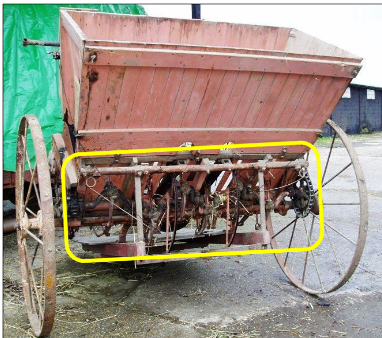
Fig.6.6 Underside of a portable trusser – Highlighted area will require guarding or use of other appropriate safety control measures
