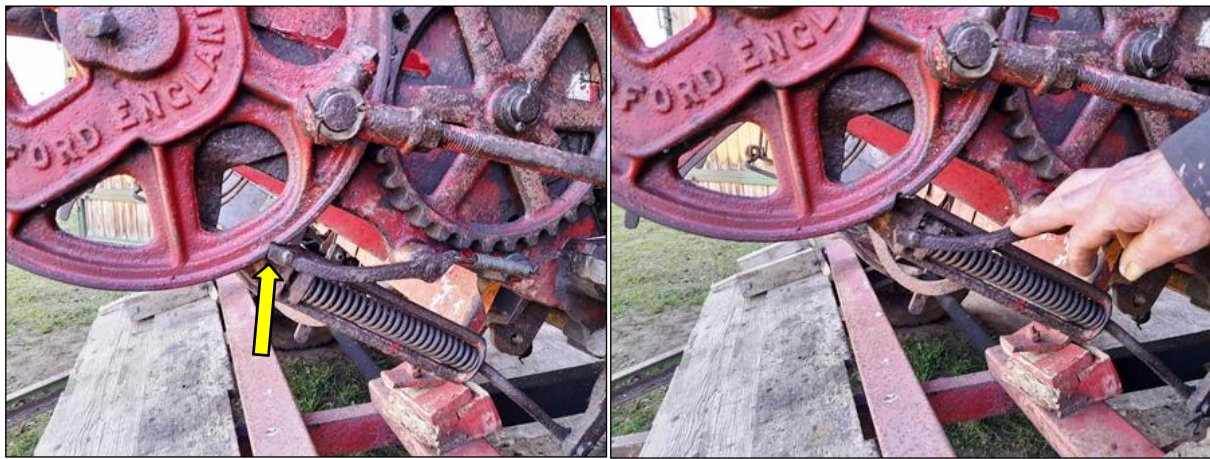
Fig.5.3 Non-return Pawl on a Howard trusser- Engaged ( left ) and disengaged ( right )
