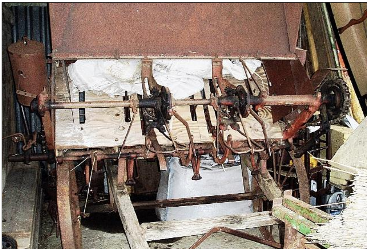
Fig.5.6 Massey-Harris double band trusser, showing arrangement of components & means of knotter shaft support.
