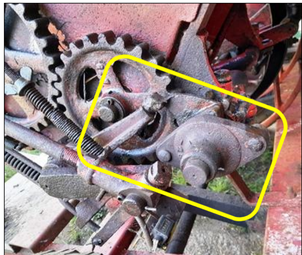
Fig.6.7 Howard trusser knotter trip & drive engagement mechanism ( highlighted )
