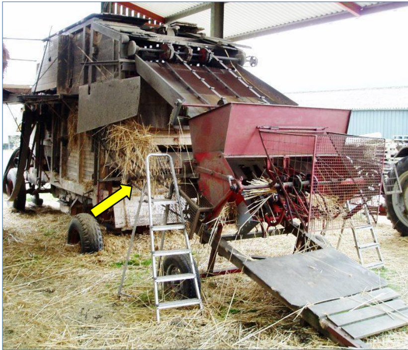
Fig.6.1 Portable trusser chain-driven from a threshing machine / reed comb
