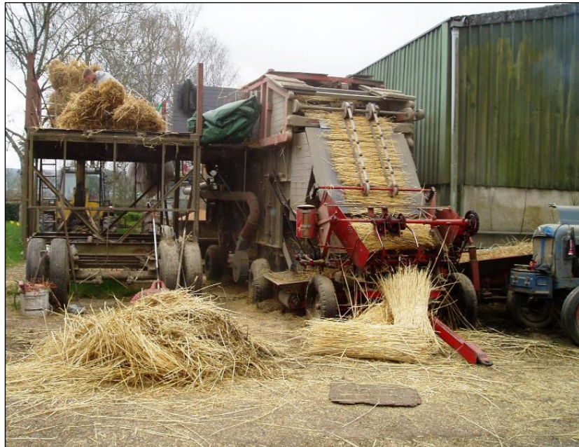
Fig.2.1 Standalone, wheeled double band trusser packaging combed wheat reed from a reed comber
