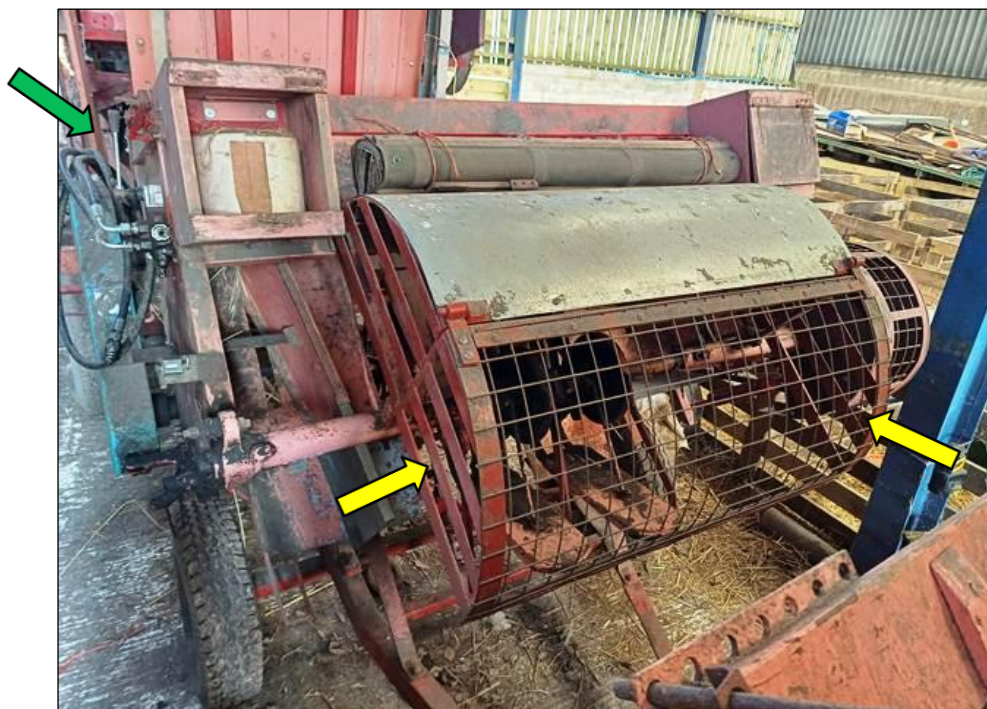
Fig.6.3 Ruston & Hornsby trusser converted to hydraulic drive with retrofit hinged steel mesh guard fitted over the Knotters and Discharge Arms
