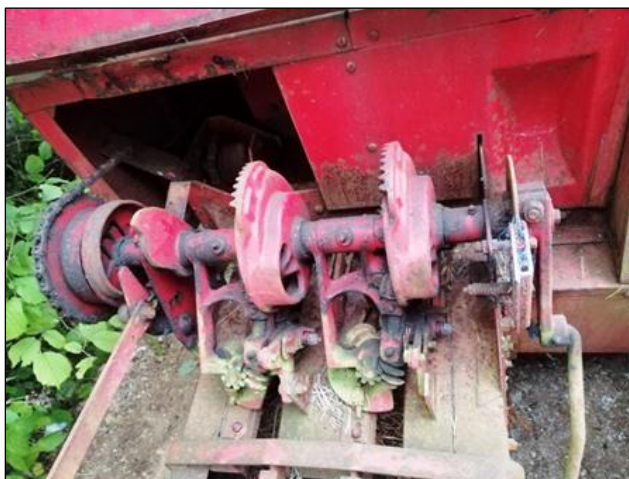
Fig.4.4 Knotter Stack on a second-hand 'spares or repair' New Holland baler
