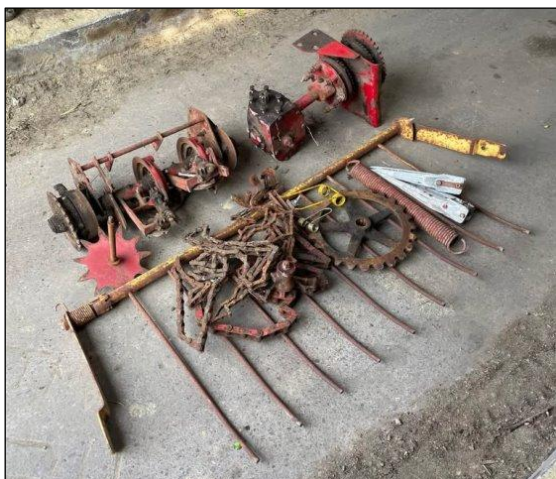
Fig.4.3 Second-hand New Holland baler parts (£150) – Knotter Stack top left
