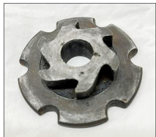
Fig.5.23 Albion binder (6-notch) Twine Disc with ratchet drive teeth on rear (upper) face
