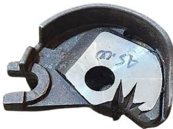
Fig.5.12 McCormick binder knotter Twine Retainer ( new, replacement part )
