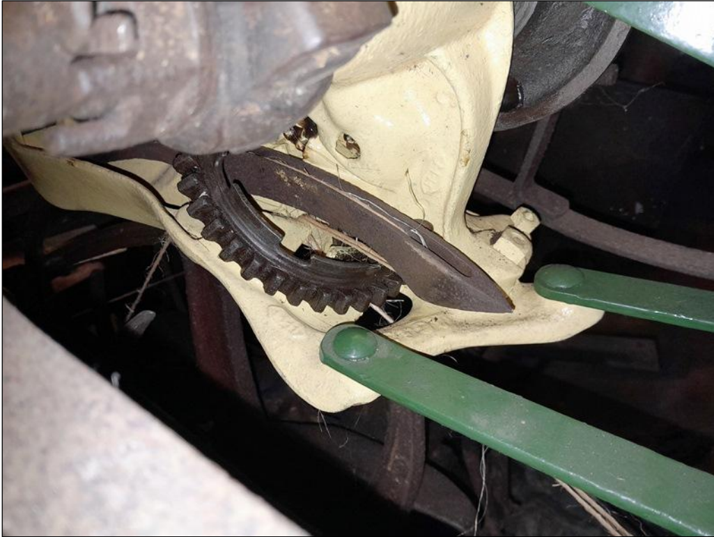
Fig.5.20 Massey-Harris binder knotter in operation – Needle drawing twine over the Twine Bridge and is about to place the strand into the waiting Twine Disc/Ring ‘notch’
