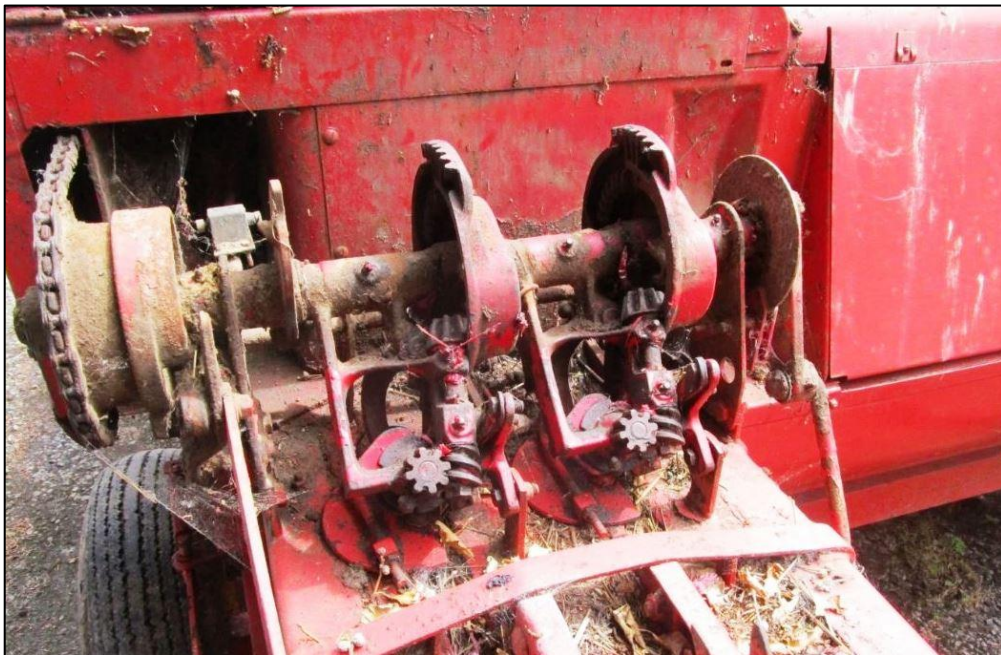
Fig.4.20 Pair of Deering-type knotters installed on a 1960s New Holland conventional baler
