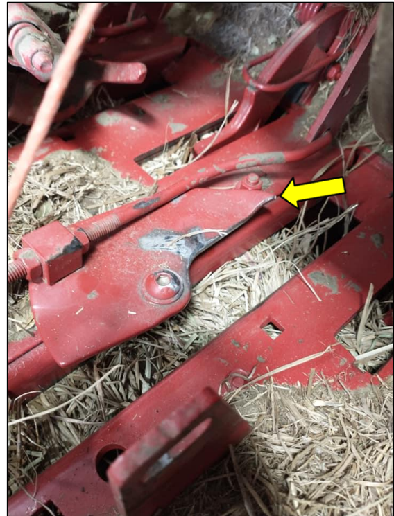
Fig.4.8 Conventional baler twine finger ( arrowed ) in open position
