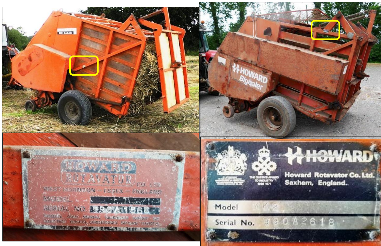
Fig.4.4 Howard Bigbaler serial number plate locations ( highlighted ) and example plates - Mk1/1a ( left ) and Mk2 ( right )
