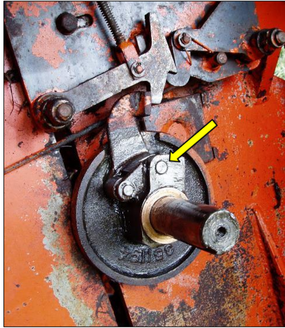
Fig.6.6 Knotter trip arm assembly – Trip arm pivot pin (arrowed)
