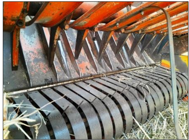
Fig.5.10 The finished job - Modified Bigbaler 'throat' ribs: Note the reduction in rib height but retention of the original rib profile ( above & right )
