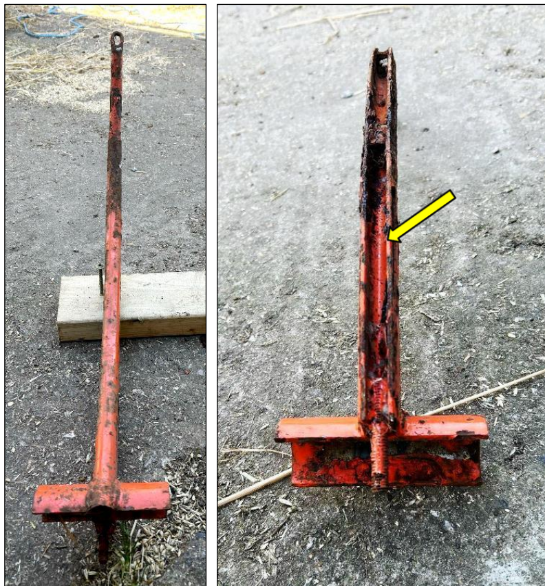
Fig.6.16 Bigbaler Mk1/1a Needle – upper surface (left) and underside (right) showing channel for passage of twine (arrowed)
