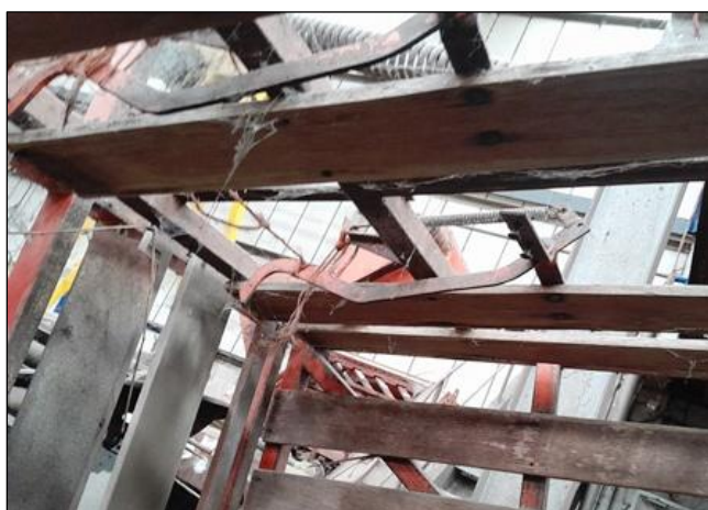
Fig.5.15 Roof Hooks tied-up so as not to contact bale
