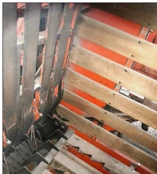
Fig.5.17 Spaced wooden slats on bale chamber sides – Mk1 & early-Mk2 Bigbalers
