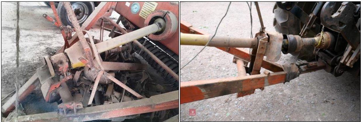
Fig.5.27 Bigbaler two-section p.t.o. shafts with mid-support bearing & pedestal: - Fixed pedestal type ( retrofit ) on Mk1 baler ( left ) - ( N.B. Front p.t.o. shaft section not fitted) - Pivoting pedestal type on Mk2 Bigbaler ( right )
