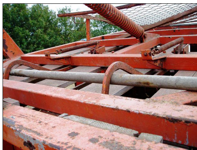
Fig.5.16 Roof Hooks disengaged by use of a broom handle ( N.B. Broom Head is optional)
