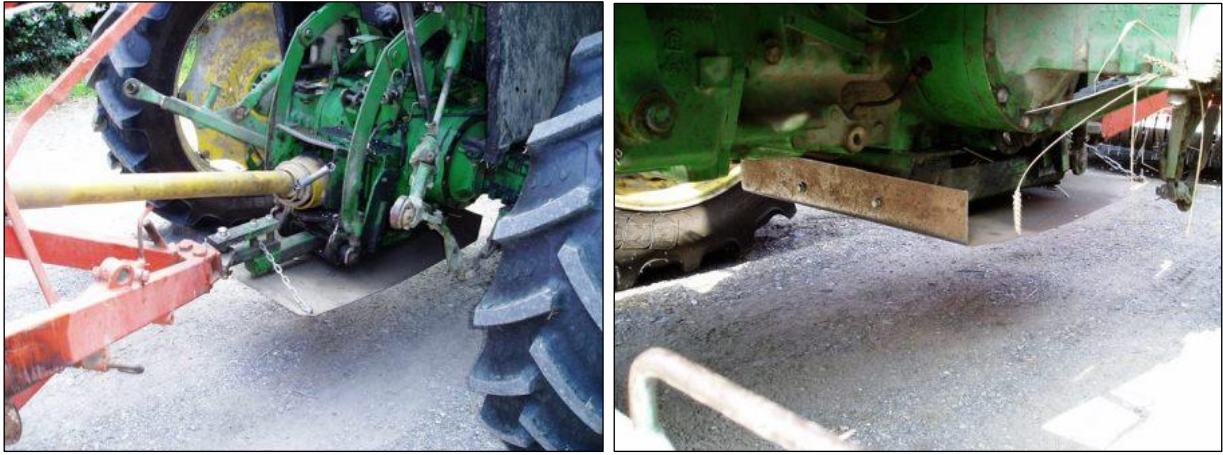
Fig.7.2 Steel 'belly plate' fitted under the tractor's drawbar/pick-up hitch assembly
