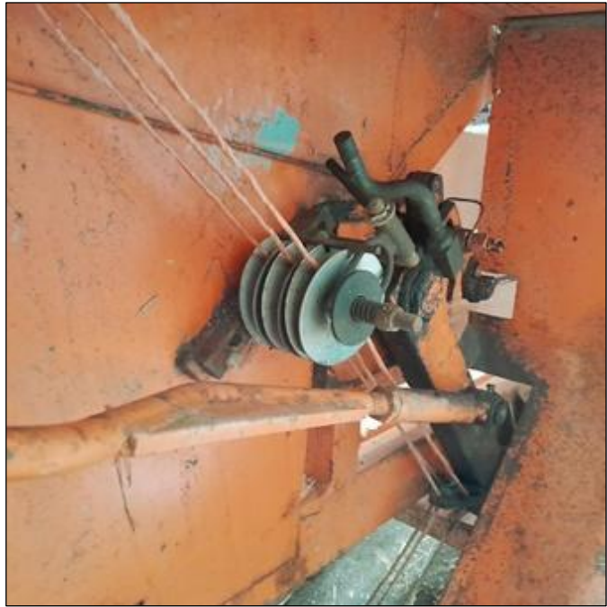
Fig.6.33 Disc-type twine tensioners – Mk2 Bigbaler
