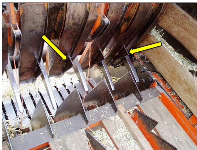
Fig.5.12 Packing plate triangular 'crop lifters' (arrowed)
