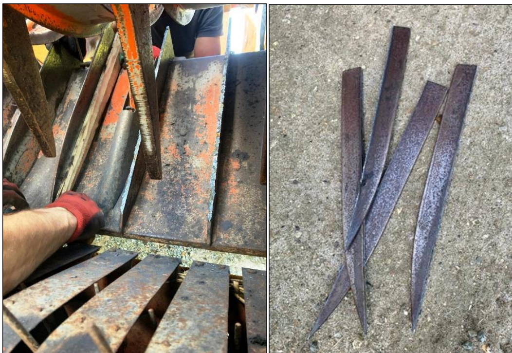
Fig.5.9 Modifying the 'throat' rib height and profile of a Mk1a Bigbaler Use of a wooden template to guide the ( plasma ) cutting torch ( left ) and the resulting rib offcuts ( right )
