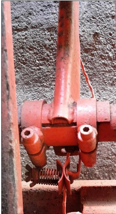
Fig.6.31 Different twine tensioner mounting locations and twine routings used on Mk1 & Mk1a Bigbalers - Mk1 ( left ) and Mk1a ( above )
