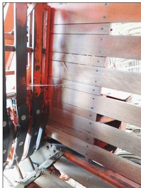
Fig.5.18 Gaps between bale chamber side boards in-filled ( as standard ) – later-Mk2 Bigbaler
