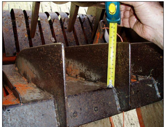
Fig.5.7 Perpendicular height of an unmodified 'throat' rib where it enters the bale chamber (~115 mm)
