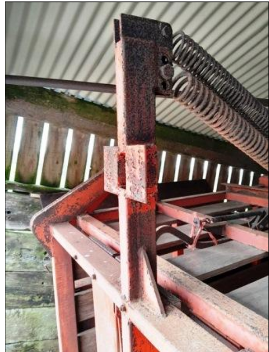
Fig.5.22 Mk2 Bigbaler tailgate spring mounting post extended to increase the mechanical advantage of the springs
