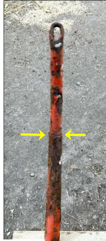
Fig.6.17 Bigbaler Mk1/1a Needle – side view ( above ) and tip detail ( right ). Point of change in needle section width ( arrowed )
