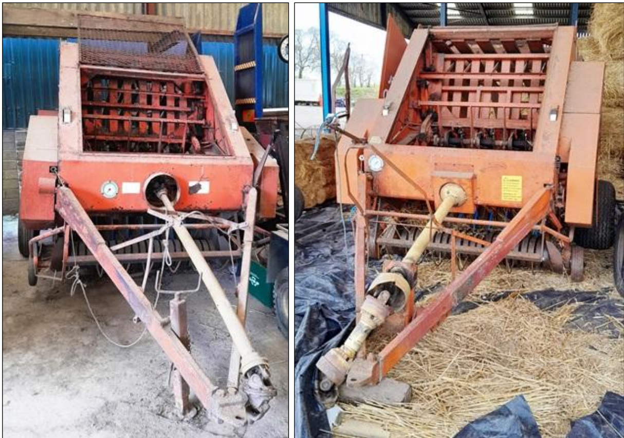
Fig.5.25 Bigbaler p.t.o. drivelines: Mk1 Bigbaler single-section shaft with wide-angle universal joint ( left ) and Mk2 Bigbaler two-section shaft with pivoting mid-support ( bearing ) pedestal ( right )
