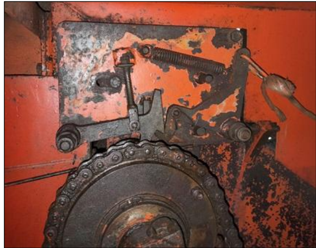
Fig.6.26 Bigbaler Knotter Trip Plate
