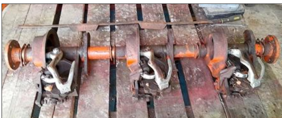
Fig.6.3 Bigbaler knotter stack - Installed ( left ) and following removal ( right & below ) - Note ready access to knotters & twine finger mechanisms following removal
