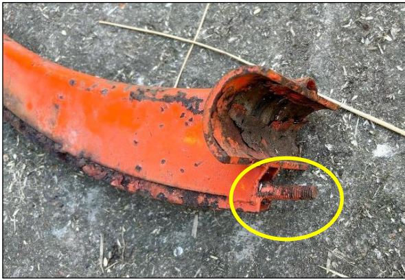
Fig.6.20 Mk1/1a Needle mounting / adjusting stud ( above - circled ), secured to plate on underside of Needle Frame ( right - arrowed )
