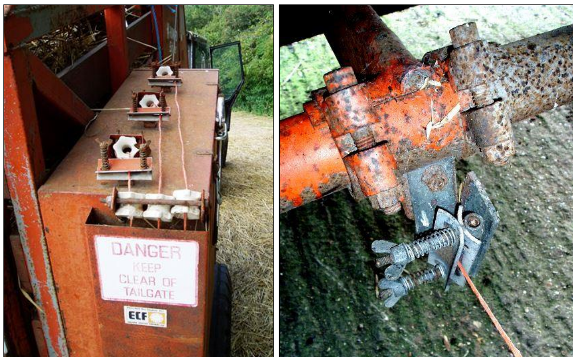
Fig.6.30 Bigbaler Mk1/1a ( adjustable ) plate-type twine tensioners – on top of twine box ( left ) & behind needles ( right )
