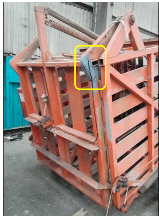
Fig.5.20 Stronger/heavier Mk2 Bigbaler tailgate featuring two counterbalance springs. In-service reinforcement of tailgate frame ( highlighted )
