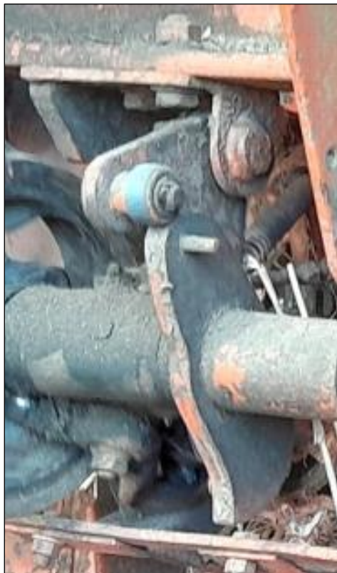
Fig.6.27 Twine Finger Cam Roller - Correct 'at-rest' position on the operating cam
