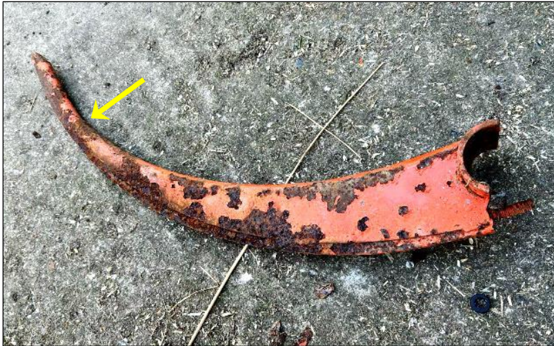
Fig.6.17 Bigbaler Mk1/1a Needle – side view ( above ) and tip detail ( right ). Point of change in needle section width ( arrowed )
