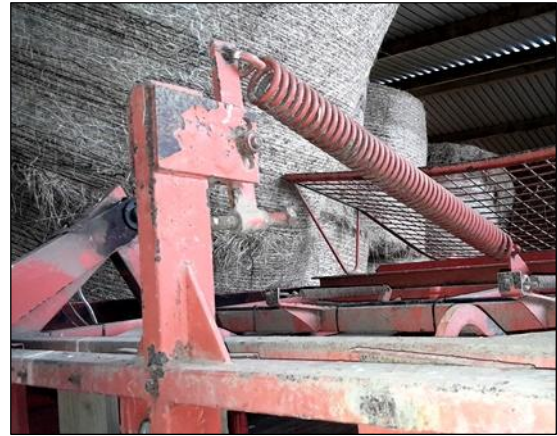
Fig.5.21 Adjustable ( single ) tailgate spring as fitted to later Mk2 Bigbalers
