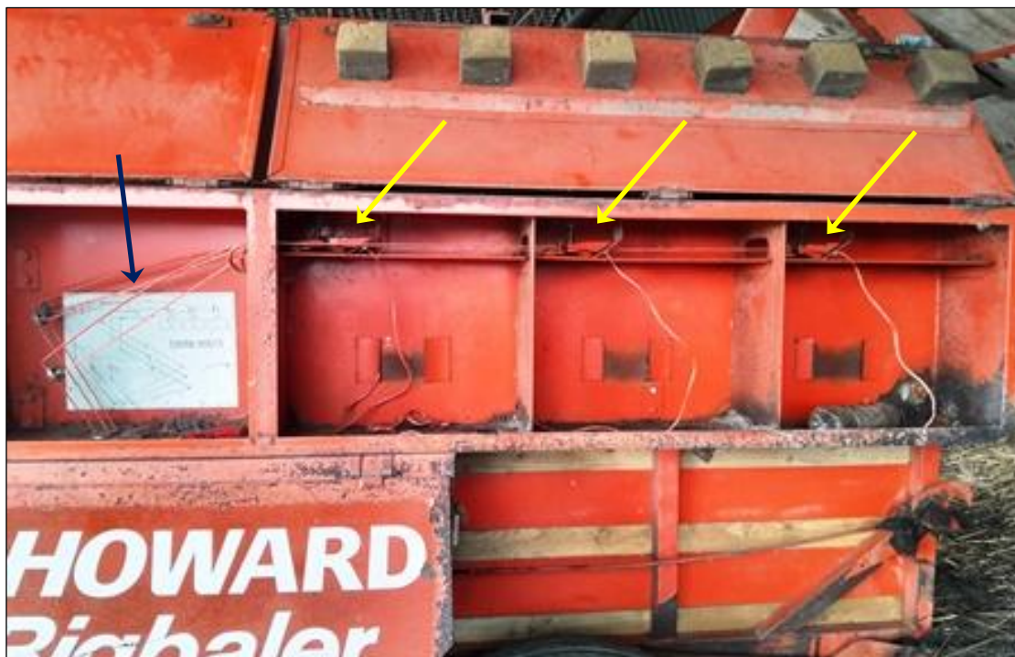
Fig.6.34 Bigbaler Mk2 twine box featuring plate-type twine tensioners (Yellow arrows) and spring arm twine guides (Blue arrow)
