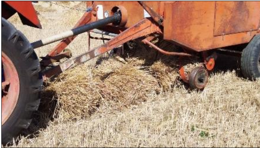
Fig.8.2 Mk1a Bigbaler baling thatching straw – Pick-up reel & windguard operation
