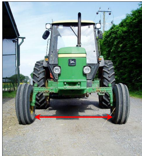
Fig. 7.1 Set the tractor's wheel track to a wide setting (at least 5 ft (1.5 m) between the tyres)
