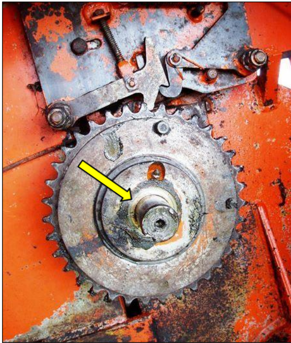
Fig.6.5 Knotter shaft sprocket & 'dish' – Central brass bush (arrowed)
