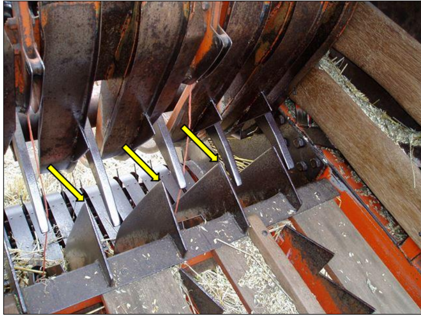
Fig.5.6 The relative positions of the packing fingers and 'throat' ribs at the top of the packing fingers' stroke. The rib front corners ( arrowed ) act as a non-return valve in the crop flow
