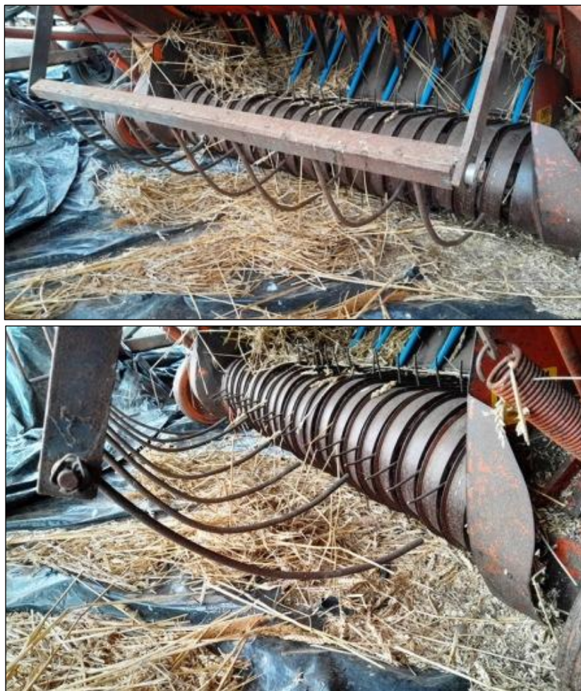
Fig.5.4 Pivoting windguard on a Bigbaler pick-up reel – Optimum design featuring long, curved tines and a low front pivot point. Pivot should ideally be spring-loaded and incorporate a travel limit-stop
