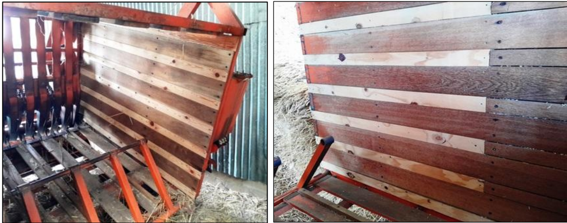
Fig.5.19 Gaps between bale chamber sides in-filled along entire length of chamber: - Mk1 Bigbaler ( left ) and later-Mk2 Bigbaler ( right )
