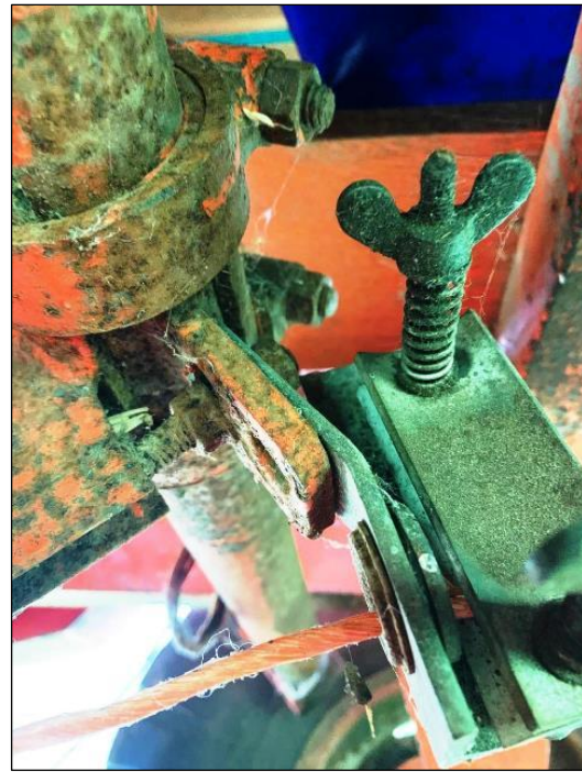
Fig.6.31 Different twine tensioner mounting locations and twine routings used on Mk1 & Mk1a Bigbalers - Mk1 ( left ) and Mk1a ( above )
