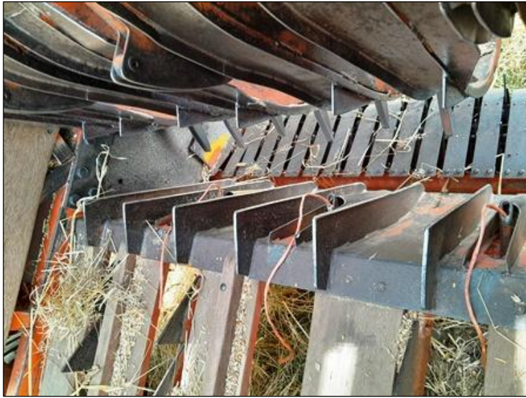
Fig.5.10 The finished job - Modified Bigbaler 'throat' ribs: Note the reduction in rib height but retention of the original rib profile ( above & right )
