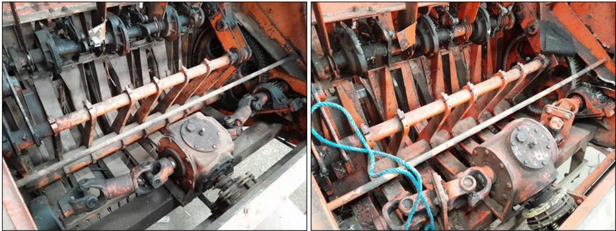
Fig.5.26 Bigbaler gearboxes and output (half) shafts: Mk1 ( left ) and Mk2 Bigbaler ( right ). Note failsafe guards fitted around Mk2 baler halfshafts
