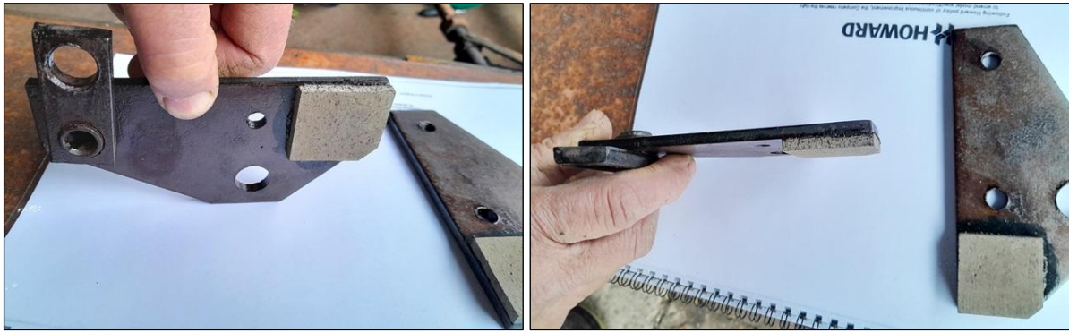
Fig.6.25 Re-lined Bigbaler knotter brake pads ( Replacement lining thickness = ~4.0 mm )
