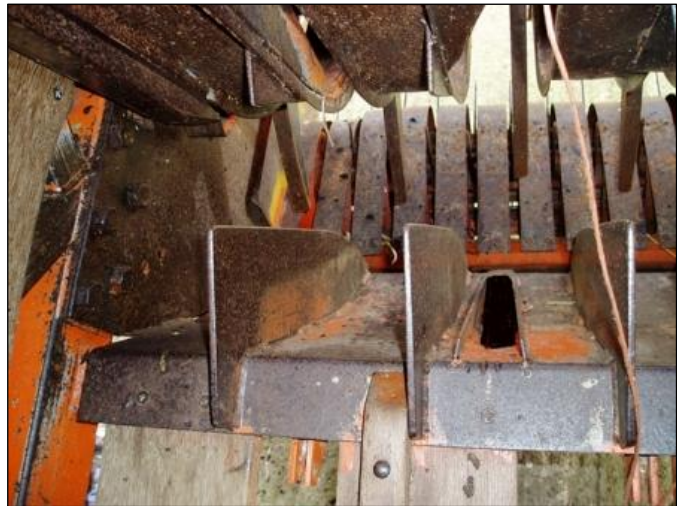
Fig.5.5 Unmodified steel ribs inside the Bigbaler's crop intake 'throat' ( viewed from inside the bale chamber )
