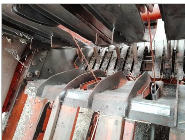
Ribs cut down towards bale chamber & upper corners rounded-off, but lower ends untouched - (Not Ideal)
