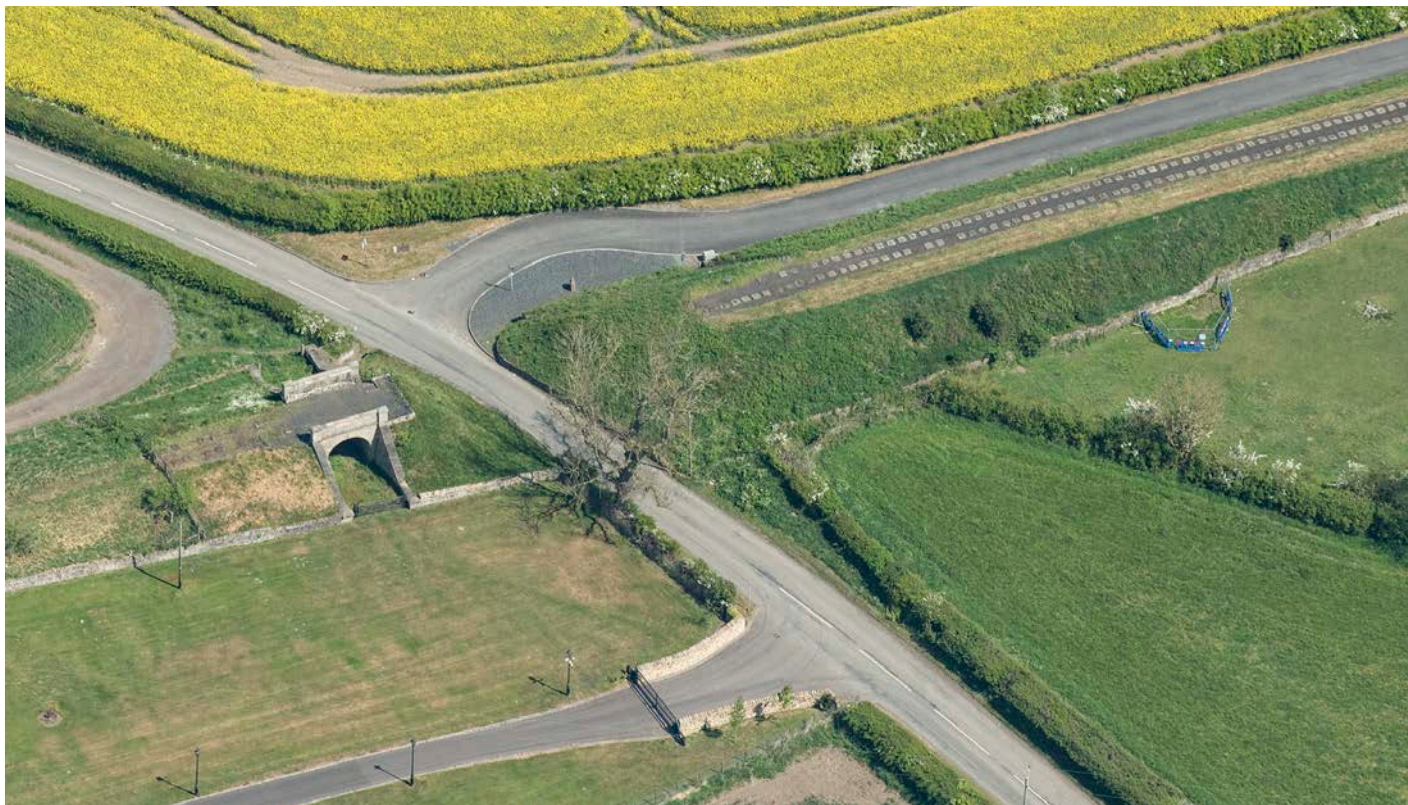
Above: Modern imagery is useful for condition assessment of the railway. This section of the Brusselton West Incline shows the 1833 accommodation bridge , boundary walls and excavated sleeper stones. Another underbridge once carried the railway over the road, but this was demolished in 1954. 34340_036 12-MAY-2025 © Historic England Archive
