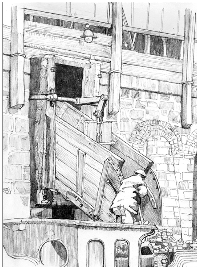
Figure 6: Reconstruction drawing of a locomotive taking on coal using the hopper/chute mechanism, based on historic photographs. Allan T Adams © Historic England
