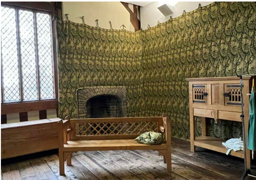
Figure 21: Traditional methods of reducing heat loss from the occupants to the building envelope included the use of hanging fabrics (top), panelling and shutters (bottom). © Tobit Curteis Associates
