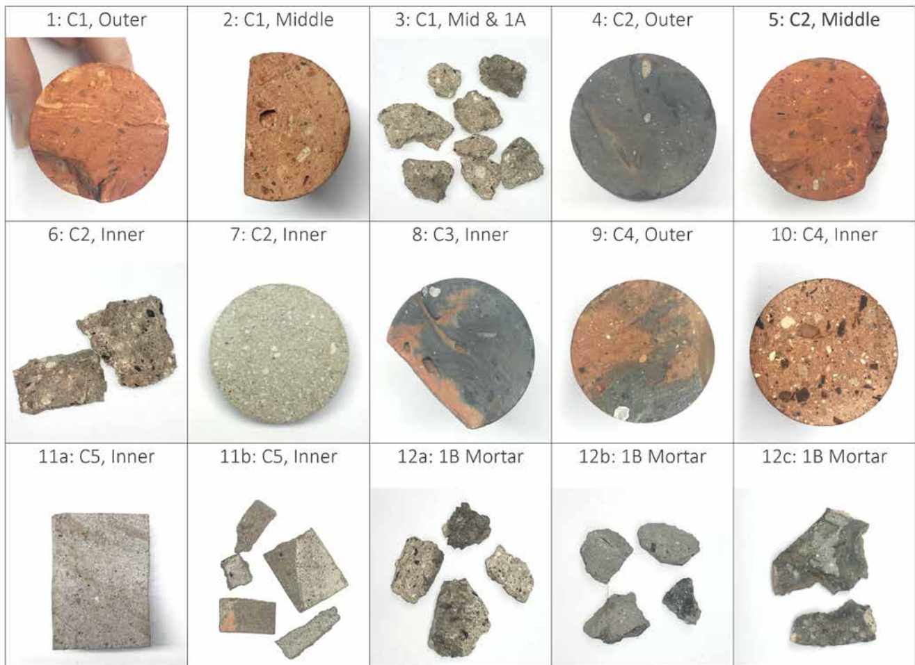
Figure 9: Photographs of material samples tested. Nine samples were selected for full characterisation of density, absorption coefficient, saturation water content and reference water content: seven brick samples from cores C1-C4 (numbers 1, 2, 4, 5, 8, 9 and 10); one plaster sample (number 7); one modern mortar joint sample (number 11). Five sets of original mortar fragments were selected for partial characterisation of density, saturation water content and reference water content (numbers 3, 6, 12a, 12b and 12c). © Greengauge.
