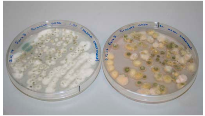
Figure D7: Cultured swabs from before and after cleaning with 1.2% hydrogen peroxide: on granite.
