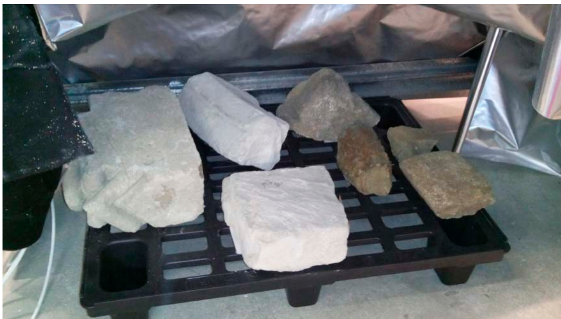
Figure D10: UVC trial set-up. Pallet with stones that have been brush vacuumed and are awaiting UVC treatment.
