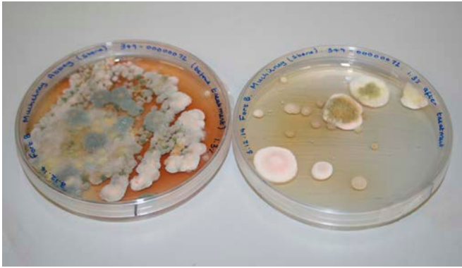
Figure D6: Cultured swabs from before and after cleaning with 1.2% hydrogen peroxide: on limestone.
