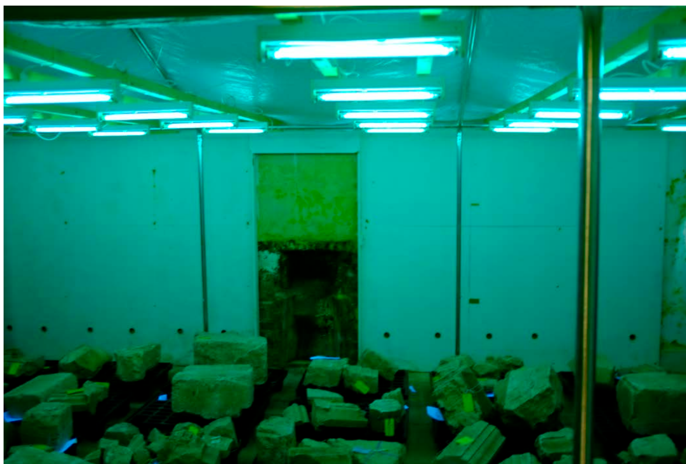
Figure D11: Stones being irradiated with UVC bulbs fitted to the marquee frame.
