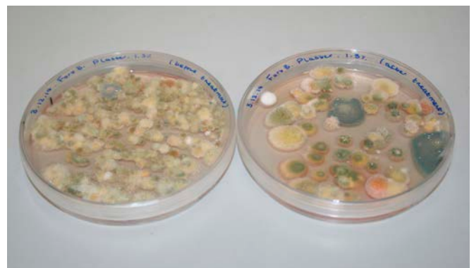
Figure D9: Cultured swabs from before and after cleaning with 1.2% hydrogen peroxide: on plaster.
