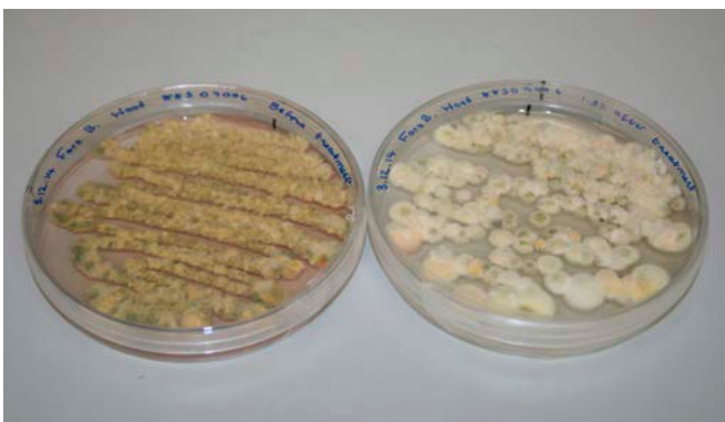
Figure D8: Cultured swabs from before and after cleaning with 1.2% hydrogen peroxide: on wood.
