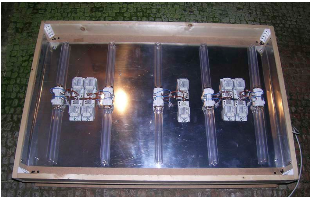
Figure C1: The UVC box designed and built for the initial trials is shown here upside-down. The inside of the box was lined with polished aluminium sheet, to reflect maximum radiation from the lamps onto the mosaic.
