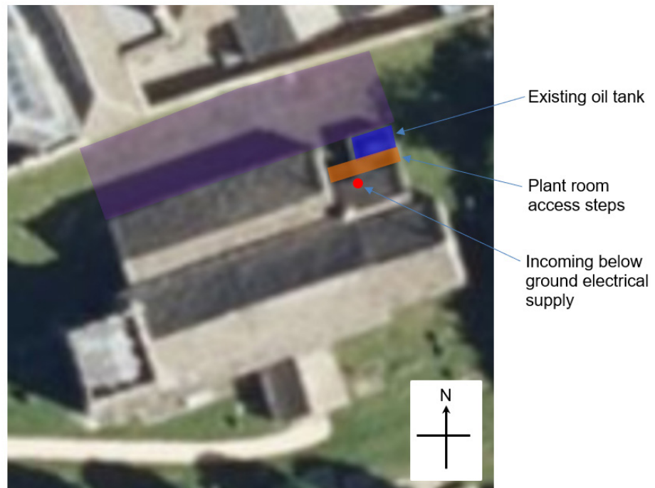
Figure 5: External plant and utilities.
