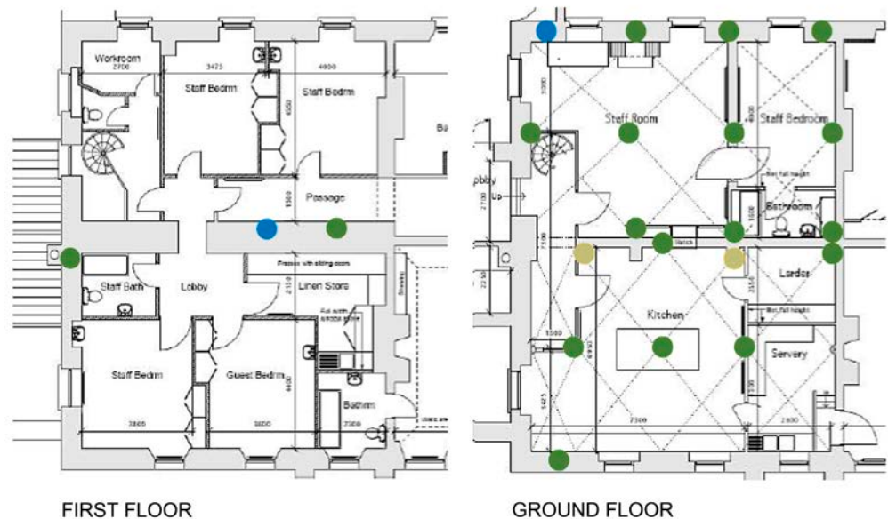
Figure 48: Ground and first floor plans showing locations of samples taken in March 2011. A drying environment was maintained by the heating system and blowers. Thermo-hygrometer readings taken around the rooms were 45% relative humidity at 13 to 15° (in three locations) on the ground floor and 45 to 54% relative humidity at 12 to 15°C (in four locations) on the first floor.
