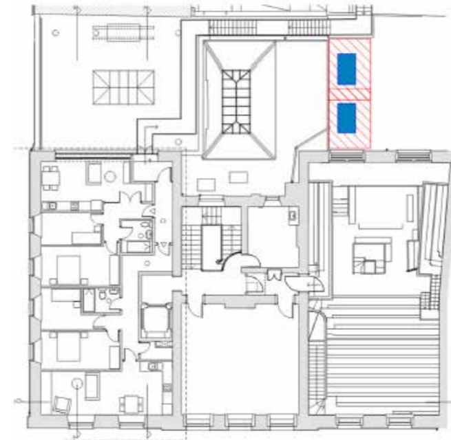
Indicative location of 2No. Clade ACER 65/50 Low Noise ASHPs
