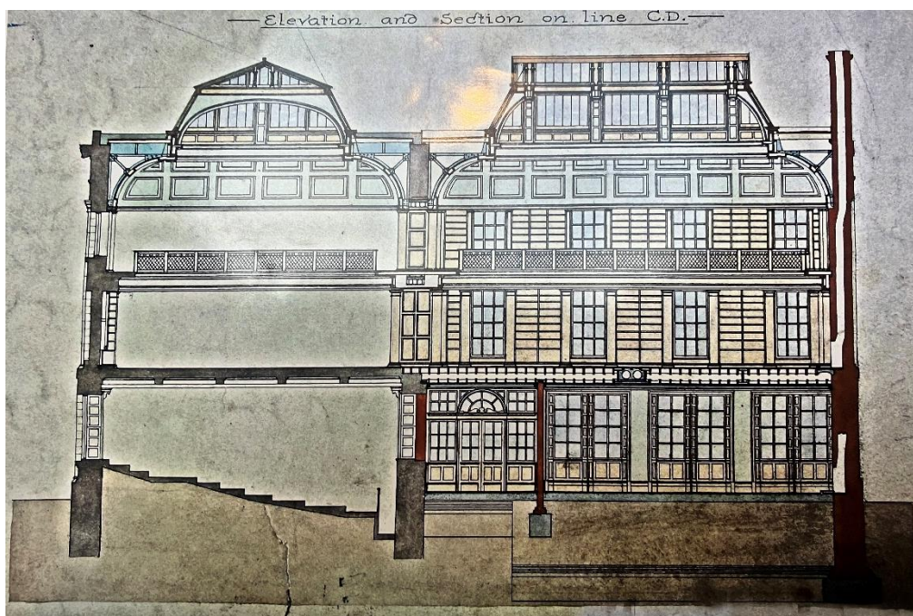
Figure 1: Archive section cut E-W through the Main Library (short section) and Reading Room (long section)
